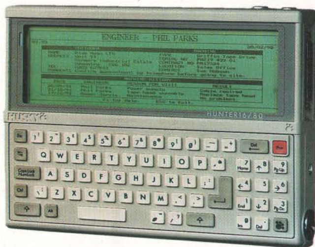
The Husky Hunter hand-held computer features a PC-standard 25-row by 80-column display.
